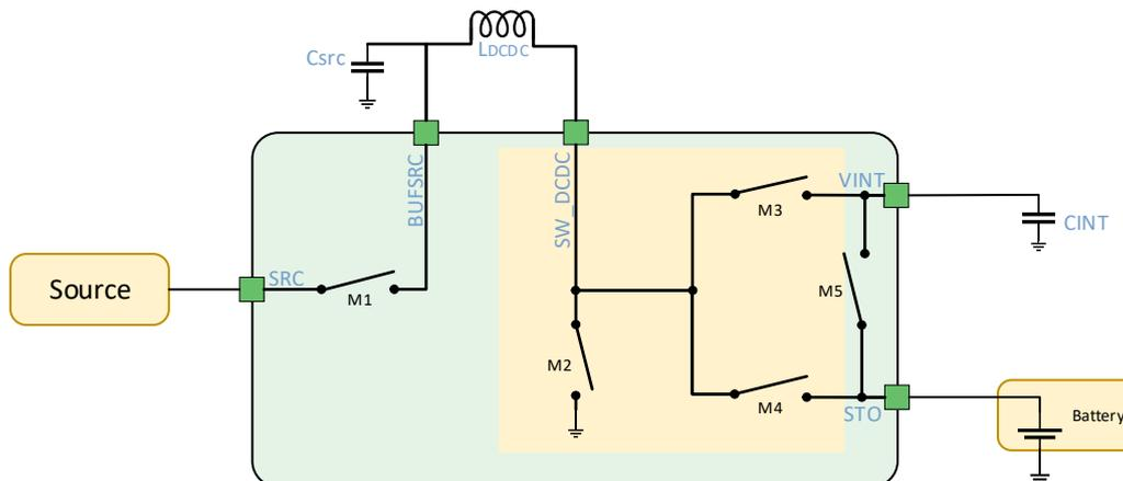
Figure 5: Simplified schematic view of the AEM10900
