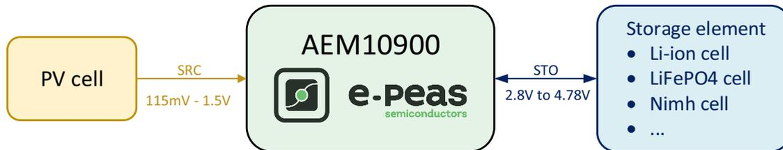
Figure 1: Simplified schematic view
