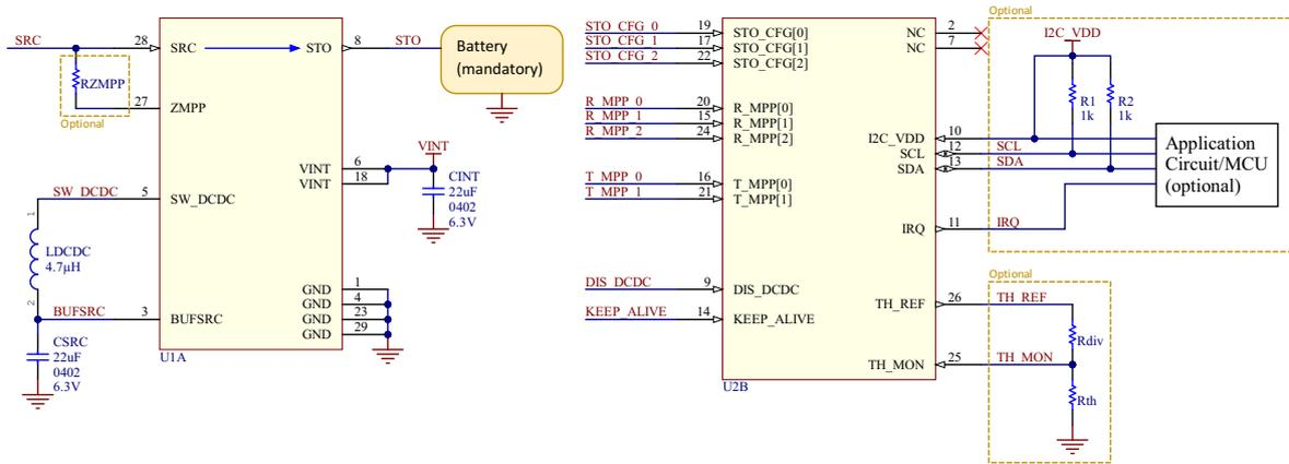
Figure 23: AEM10900 schematic
