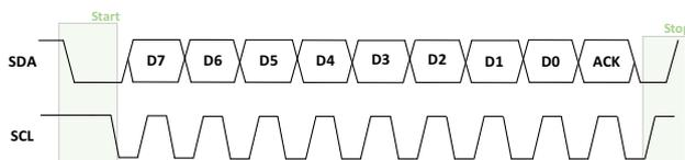
Figure 8: I<sup>2</sup>C transmission frame
